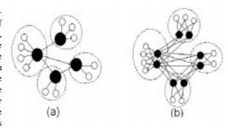
Figure 1: Illustration of a super-peer network (a) with no redundancy, (b) with 2-redundancy. Black nodes represent super-peers, white nodes represent clients. Clusters are marked by the dashed lines.
