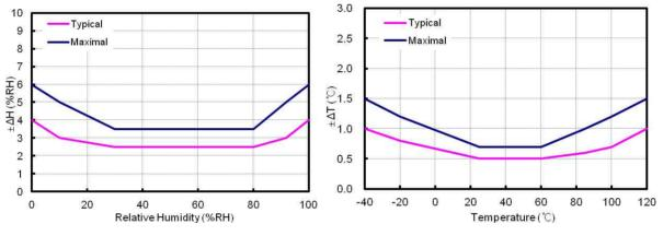
Fig.1 Humidity-accuracy at 25  $^\circ\!\!\!{\rm C}$
