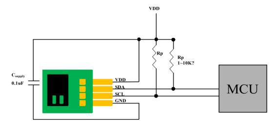
Fig.10 HT-01D I<sup>2</sup>C Interface
